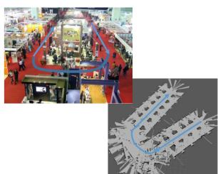
Grid Mapping adapted from Hector Mapping code which uses Hokuyo laser range finder and IMU sensors
